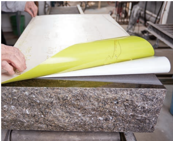
Apply to Stone: Clean, smooth cuts and support for center of letters and numbers.
